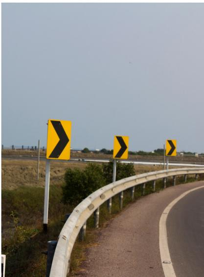
The Township of Malahide requested the installation of guard rails on Imperial Road in the Village of Port Bruce. In response, Council instructed staff to install Chevron alignment signs on the road instead, based on the Ontario Traffic Manual, along the horizontal roadway curve immediately north of Rush Creek Line.
