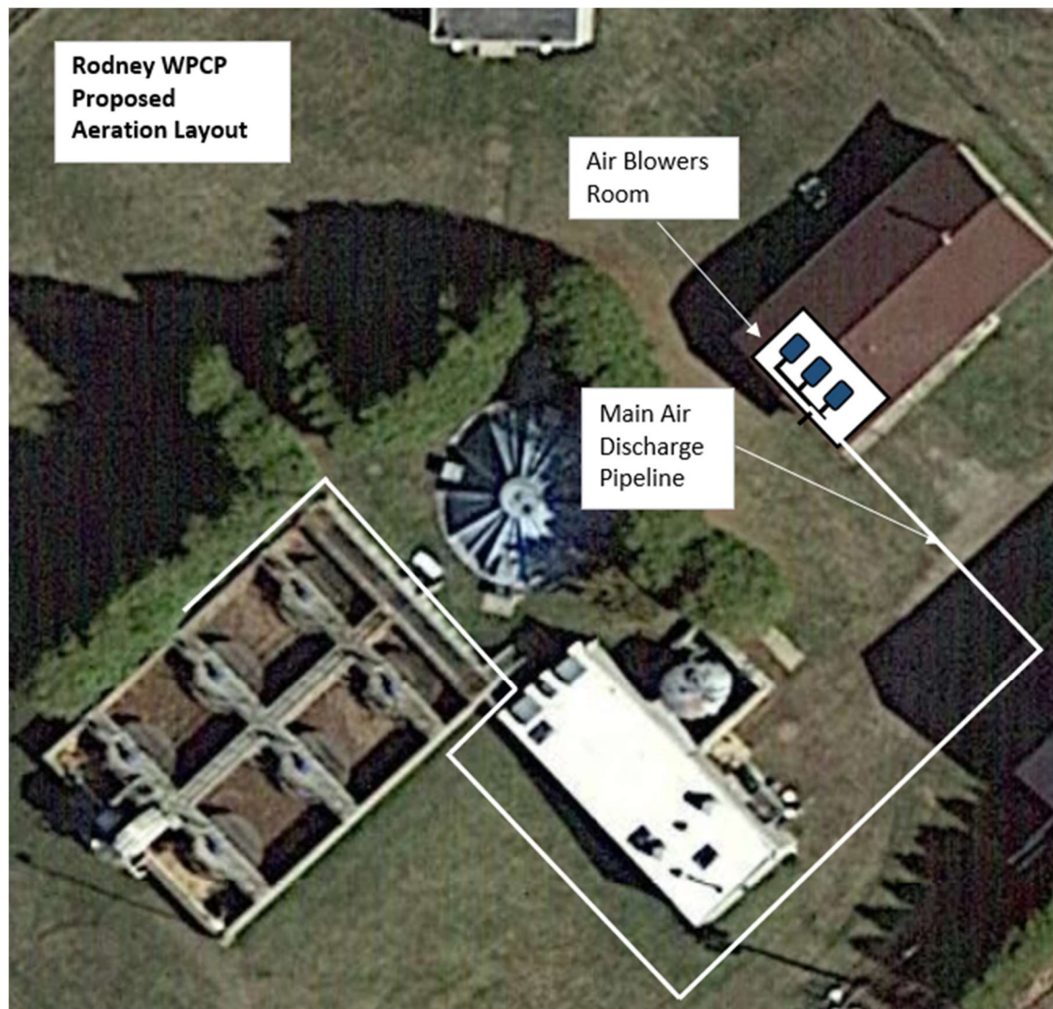
Figure 6.1 – Air Blowers and Main Air Discharge Pipeline Layout.
